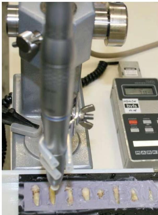
**Fig. 1.** Teeth embedded in a silicone model with a built-in water reservoir. IOA system hand-piece fixed at a 90° angle to the intended line of perforation, using the specially designed splint with a pressure-calibrated support plate.
